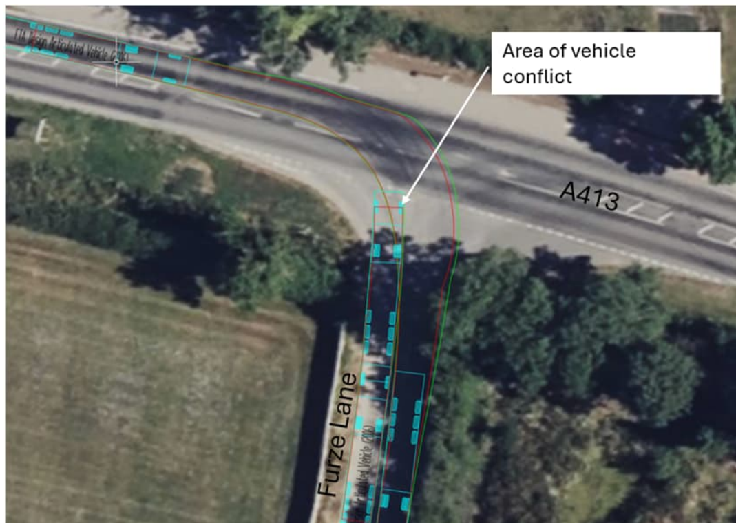
Figure 7: A413 / Furze Lane Junction HGV Swept Path
